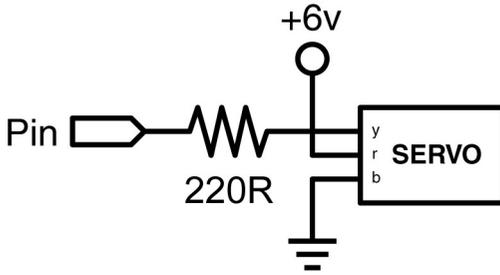
Hobby servos are a type of self-contained motor that can move in a 180° arc. All that is needed is a pulse sent every 20ms. This example uses a servoPulse function to move the servo from 10° -170° and back again.
