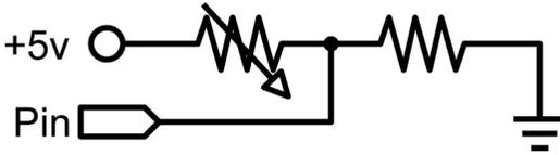
Variable resistors include CdS light sensors, thermistors, flex sensors, and so on. This example makes use of a function to read the analog value and set a delay time. This controls the speed at which an LED brightens and dims.
