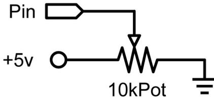
Using a potentiometer and one of the Arduino's analog-to-digital conversion (ADC) pins it is possible to read analog values from 0-1024. The following example uses a potentiometer to control an LED's rate of blinking.
